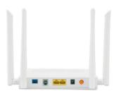
Optical Network Terminal (ONT) to receive data via optical fibre
